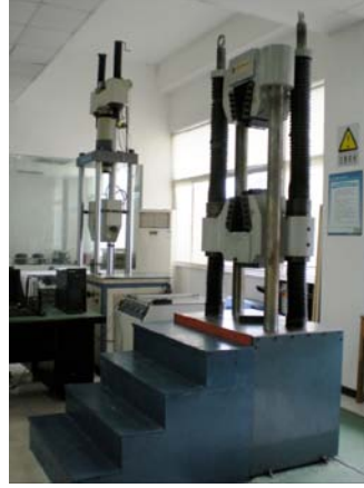
Tensile Testing Machine for PC Strand.
